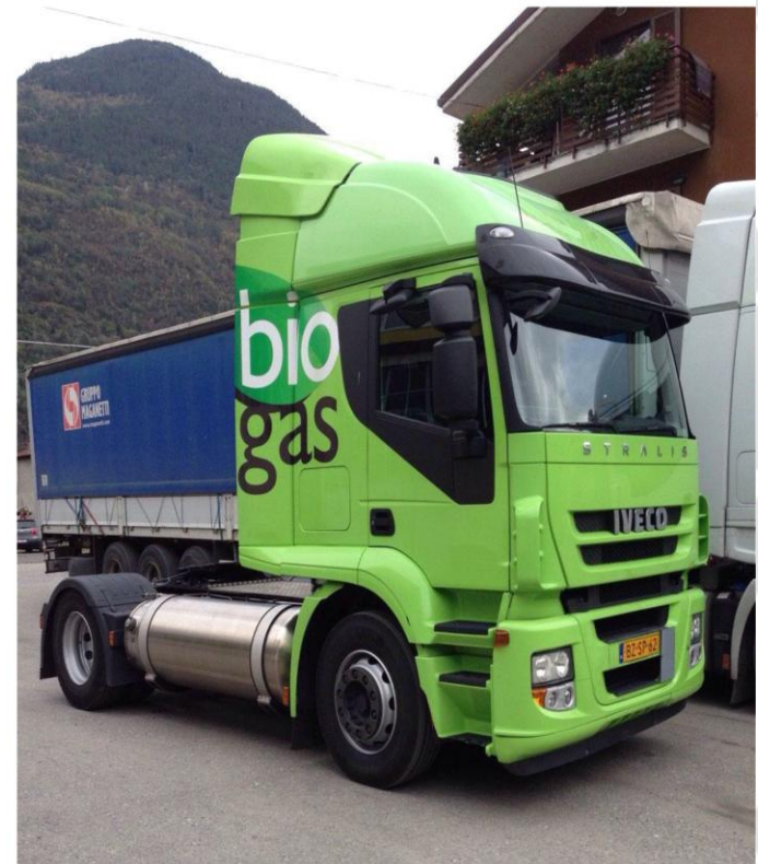
Tresenda in Teglio ( SO ), 2015 Iveco Stralis LNG Truck : test di autonomia
